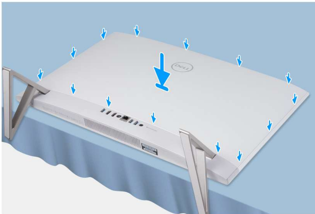
Figura22. Instalar a tampa traseira
